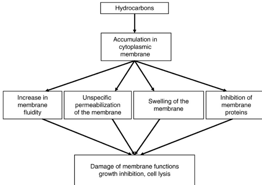
**Figure 14. Scheme of the toxicity of hydrocarbons in the cell membranes**
