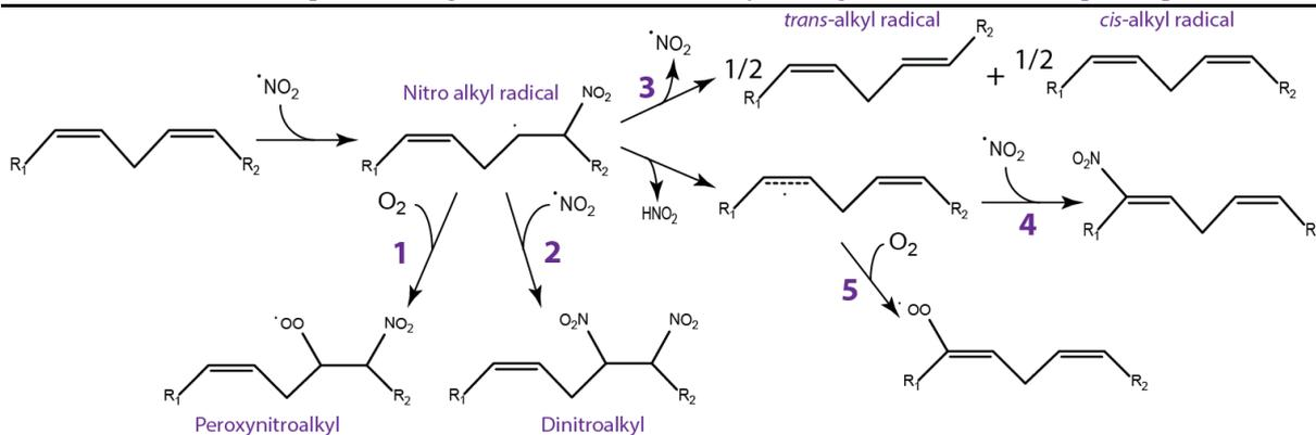
**Figure 26. Schematic representation of NO<sub>2</sub> reaction with polyunsaturated lipids**
