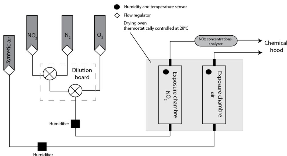
**Figure S1. Schematic representation of NO<sub>2</sub> gas delivery system**
