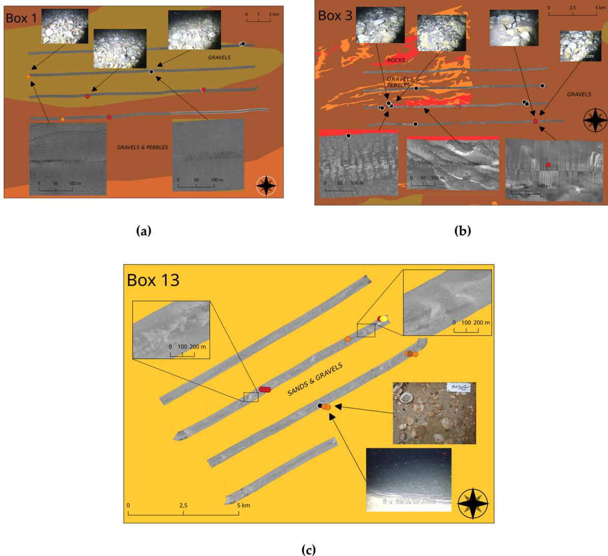
**Figure 4.** Example of scan sonar profiles collected during the VIDEOCHARM surveys in June 2010 ((a,b) boxes 1 and 3) and June 2011 ((c) box 13) with inset views for some areas of interest and snapshots of the surface sediments extracted from the ROV video footage.
