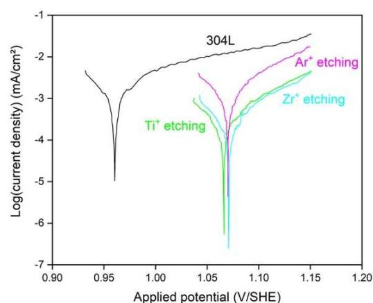
**Figure 8.** Potentiodynamic polarization curves of raw and etched 304L steel in a nitric acid solution at boiling temperature after 48 h of immersion. Black: initial 304L; violet: Ar<sup>+</sup> etching; green: Ti<sup>+</sup> etching; cyan: Zr<sup>+</sup> etching.
