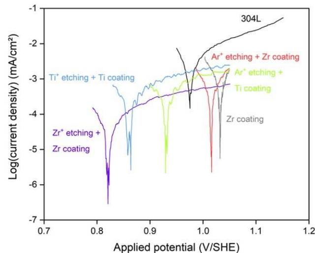
**Figure 9.** Potentiodynamic polarization curves of raw 304L and etched and metallic bond coat deposited samples in a nitric acid solution at boiling temperature after 6 h of immersion. Black: initial 304L; light green: Ar<sup>+</sup> etching + Ti coating; red: Ar<sup>+</sup> etching + Zr coating. Light blue: Ti<sup>+</sup> etching + Ti coating; deep blue: Zr<sup>+</sup> etching + Zr coating; grey: Zr coating.
