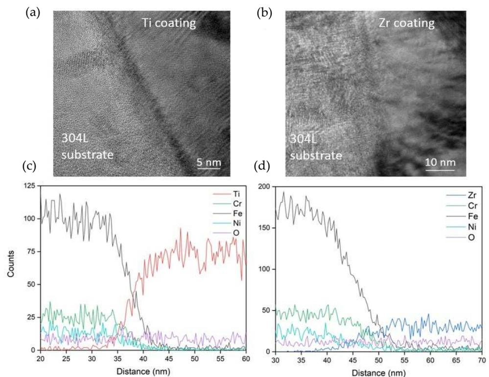
**Figure 5.** TEM observation of the substrate/metallic bond coat interface of (a)  $\text{Ti}^+$ -etched + Ti-coated and (b)  $\text{Zr}^+$ -etched + Zr-coated samples and TEM profiles for (c)  $\text{Ti}^+$ -etched + Ti-coated and (d)  $\text{Zr}^+$ -etched + Zr-coated samples.
