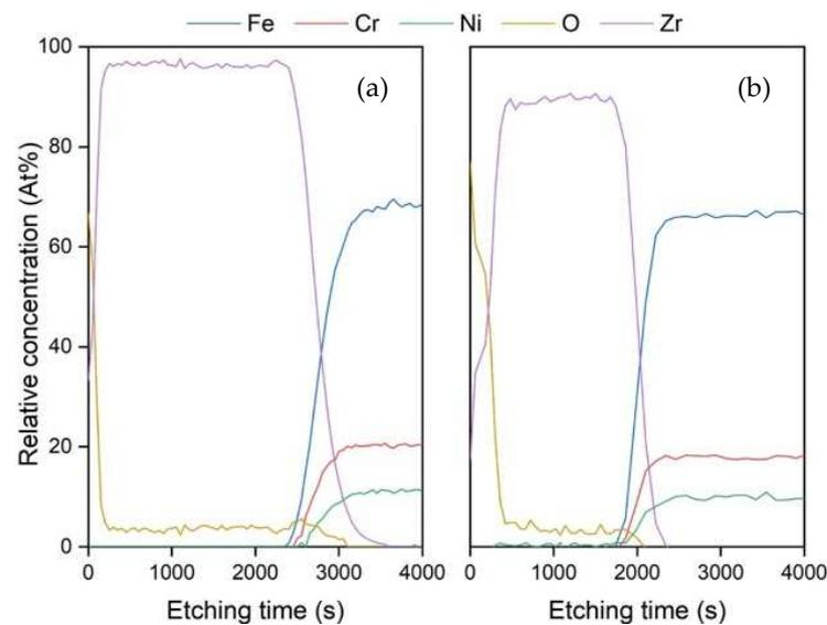
**Figure 12.** XPS depth profiles of  $Zr^+$ -etched and Zr-coated sample (a) before and (b) after 48 h of immersion in nitric acid solution at boiling temperature.
