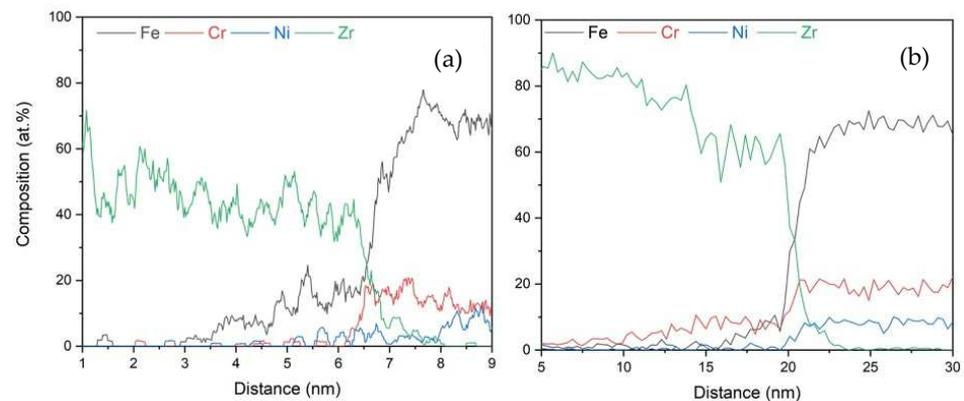
**Figure 6.** APT concentration profiles obtained for the  $Zr^+$ -etched and Zr-coated sample performed (a) in electrical mode on IRMA GPM platform and (b) in laser mode on CEA platform.
