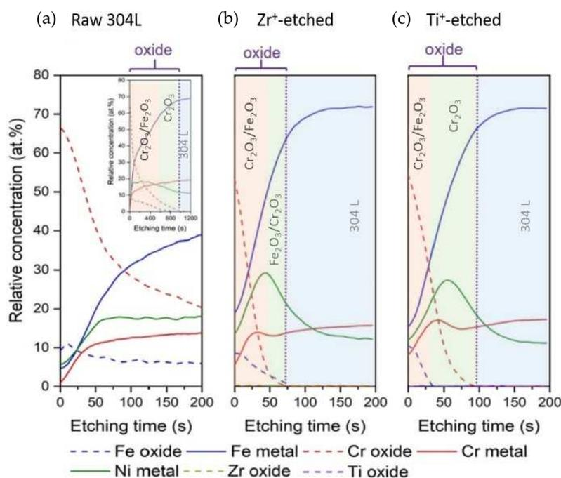
**Figure 11.** XPS depth profiles of (a) raw 304L steel and (b) Zr<sup>+</sup>- and (c) Ti<sup>+</sup>-etched samples after 48 h of immersion in nitric acid solution at boiling temperature.
