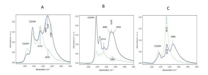
Figure 1. IR spectra of CO at 133 Pa equilibrium pressure for Mo (green line) and CoMo (thick blue line) sulfide catalysts supported on Al<sub>2</sub>O<sub>3</sub> (A), SiO<sub>2</sub> (B) and TiO<sub>2</sub> (C).
