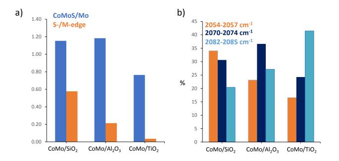
Figure 8. a) Comparison between  $MoS_2$  morphology detected for non-promoted catalysts and promotion degree obtained for promoted catalysts. b) Contribution of the three main v(CO/CoMoS) components for CoMo catalysts supported on Al<sub>2</sub>O<sub>3</sub>, SiO<sub>2</sub> and TiO<sub>2</sub>.
