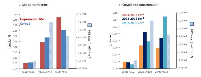
Figure 9. Comparison of a) unpromoted and promoted sites concentration, b) concentration of the 3 types of CoMoS sites with thiophene HDS rate for CoMo catalysts supported on Al<sub>2</sub>O<sub>3</sub>, SiO<sub>2</sub> and TiO<sub>2</sub>
