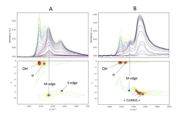
Figure 3. Spectroscopic isotherms (top) and 2D-distribution functions of the absorbances (bottom) of CO adsorbed on (A) Mo/SiO<sub>2</sub> and (B) and CoMo/SiO<sub>2</sub> catalysts.
