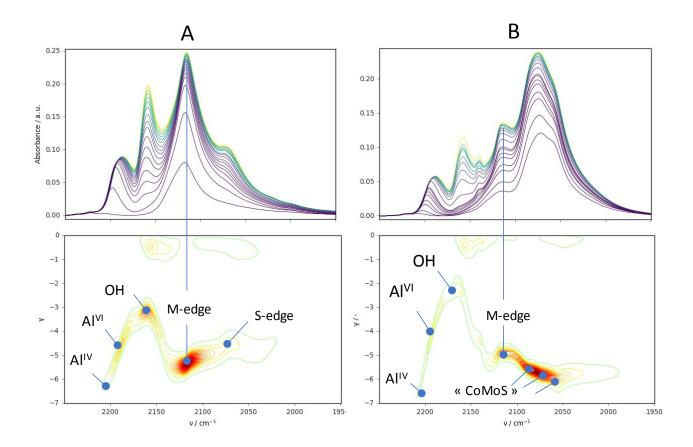
Figure 2. Spectroscopic isotherms (top) and 2D-distribution functions of the absorbances (bottom) of CO adsorbed on (A) Mo/Al<sub>2</sub>O<sub>3</sub> and (B) CoMo/ Al<sub>2</sub>O<sub>3</sub> catalysts.
