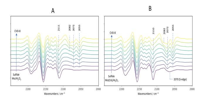
Figure 5. Second derivatives of IR spectra of CO on (Co)Mo/Al<sub>2</sub>O<sub>3</sub> catalysts prepared by CVD. (A) Co deposition on Mo/Al<sub>2</sub>O<sub>3</sub>, (B) Co deposition on Mo(CA)/Al<sub>2</sub>O<sub>3</sub>. From violet to yellow: non-promoted to Co-promoted catalysts at increasing Co content (from 0.07 to 2.32 % wt Co deposited).
