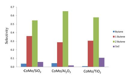
Figure 7. Percentage of different products converted in thiophene HDS reaction for CoMo catalysts supported on  $Al_2O_3$ , SiO<sub>2</sub> and TiO<sub>2</sub>
