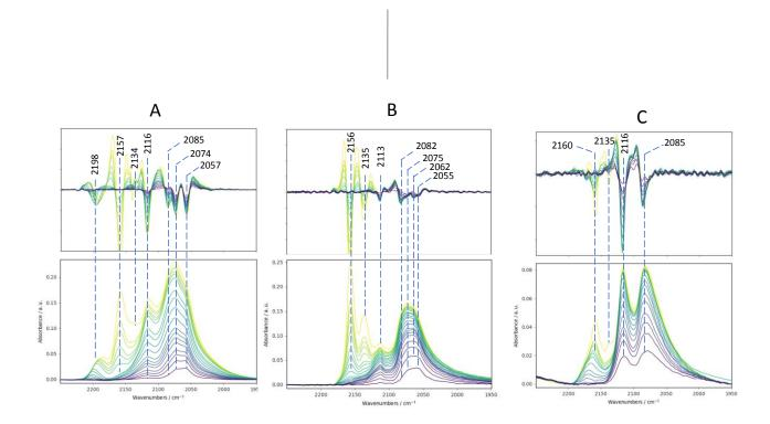
Figure 4. Bottom: IR spectra of CO adsorption from small CO doses up to saturation at equilibrium pressure (133Pa). Top: second derivative of IR spectra. A: CoMo/Al<sub>2</sub>O<sub>3</sub>, B: CoMo/SiO<sub>2</sub>; C: CoMo/TiO<sub>2</sub>
