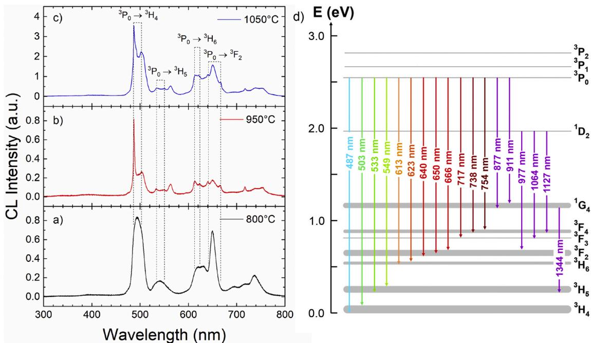
Fig. 1. CL spectra of  $\text{Pr}^{3+}$ -doped  $\text{HfSiO}_x$  thin films annealed at (a)  $800^\circ\text{C}$ , (b)  $950^\circ\text{C}$  and (c)  $1050^\circ\text{C}$  in UV-Visible range. Spectra were recorded using a probe current of 1.85 nA with an acceleration voltage of 15 kV. (d) Schematic presentation of intra-4f transitions of  $\text{Pr}^{3+}$  ions.
