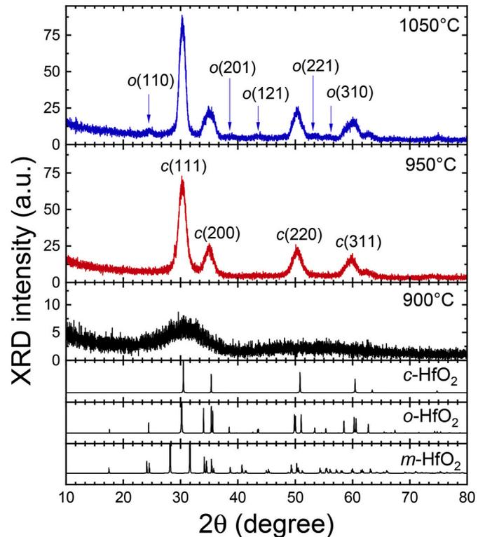
**Fig. 6.** XRD diffractogram of Pr<sup>3+</sup>-doped HfSiO<sub>x</sub> thin layers as a function of the annealing temperature. Reference pattern correspond to cubic ( $F_{m\bar{3}m}$ , JCPDS: n° 53-0550), orthorhombic ( $P_{ca21}$ , JCPDS: n° 83-0808) and monoclinic HfO<sub>2</sub> ( $P_{21/c}$ , JCPDS: n° 43-1017).
