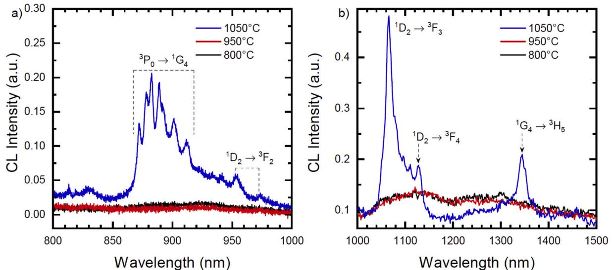
Fig. 3. CL spectra of  $\text{Pr}^{3+}$ -doped  $\text{HfSiO}_x$  thin films annealed at 800°C, 950°C and 1050°C in near IR range. Spectra were recorded using an acceleration voltage of 15 kV with (a) a probe current of 1.85 nA and (b) a probe current of 9.47 nA, by consequence measurements of intensities may differ between (a) and (b).
