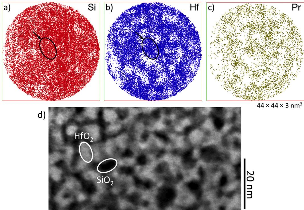
**Fig. 5.** Three dimensional mappings of (a) Si-, (b) Hf- and (c) Pr-atomic distributions obtained on Pr<sup>3+</sup>-doped HfSiO<sub>x</sub> thin layer annealed at 950°C. The surrounded area shows a part of the HfO<sub>2</sub> phase. It evidences an important artificial inclusion of Si atoms in the HfO<sub>2</sub> phase due to field effect during the APT analysis [30]. (d) STEM HAADF picture of Pr<sup>3+</sup>-doped HfSiO<sub>x</sub> film annealed at 950°C.
