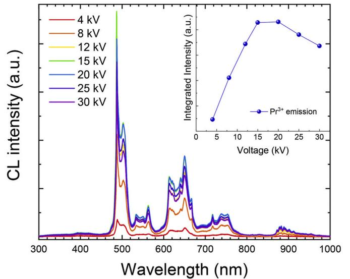
Fig. 4. CL spectra of  $\text{Pr}^{3+}$ -doped  $\text{HfSiO}_x$  thin films annealed at 1050°C measured for different acceleration voltages. Spectra were recorded using a probe current of 1.85 nA. The inset corresponds to the evolution of the integrated intensity of the  $\text{Pr}^{3+}$  signal as a function of the acceleration voltage.
