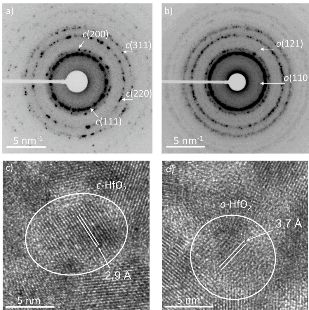
Fig. 7. (a–b) SAED patterns measured on samples annealed at  $950^\circ\text{C}$  and  $1050^\circ\text{C}$ , respectively. (c–d) High-resolution STEM images obtained on  $\text{Pr}^{3+}$ -doped  $\text{HfSiO}_x$  film annealed at  $1050^\circ\text{C}$ .
