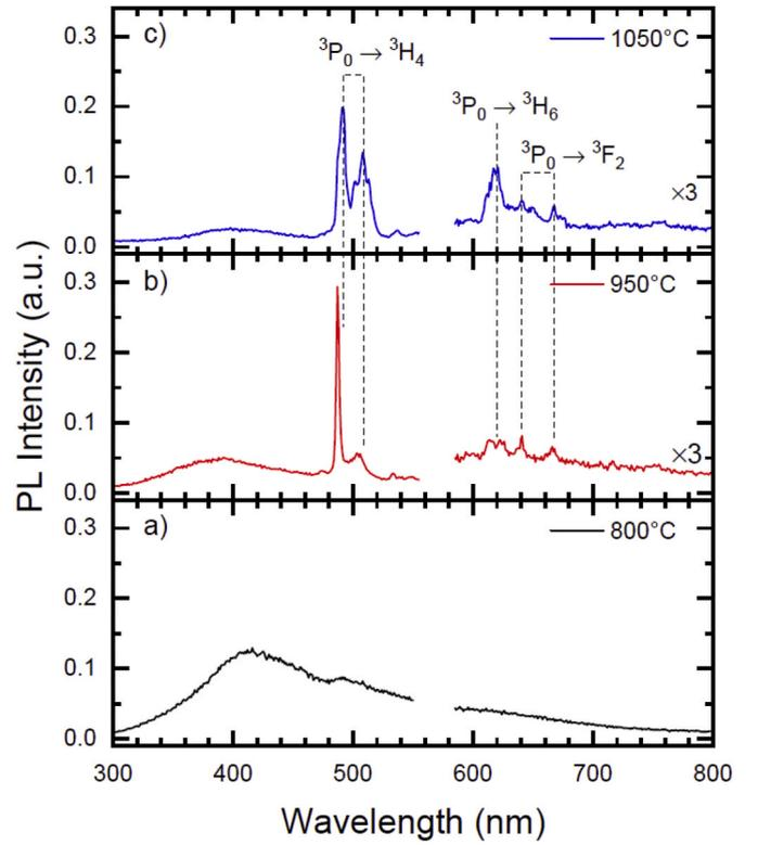
Fig. 2. PL spectra of Pr<sup>3+</sup> doped HfSiO<sub>x</sub> thin films annealed at (a) 800°C, (b) 950°C and (c) 1050°C in UV–Vis range. The excitation wavelength is 285 nm.
