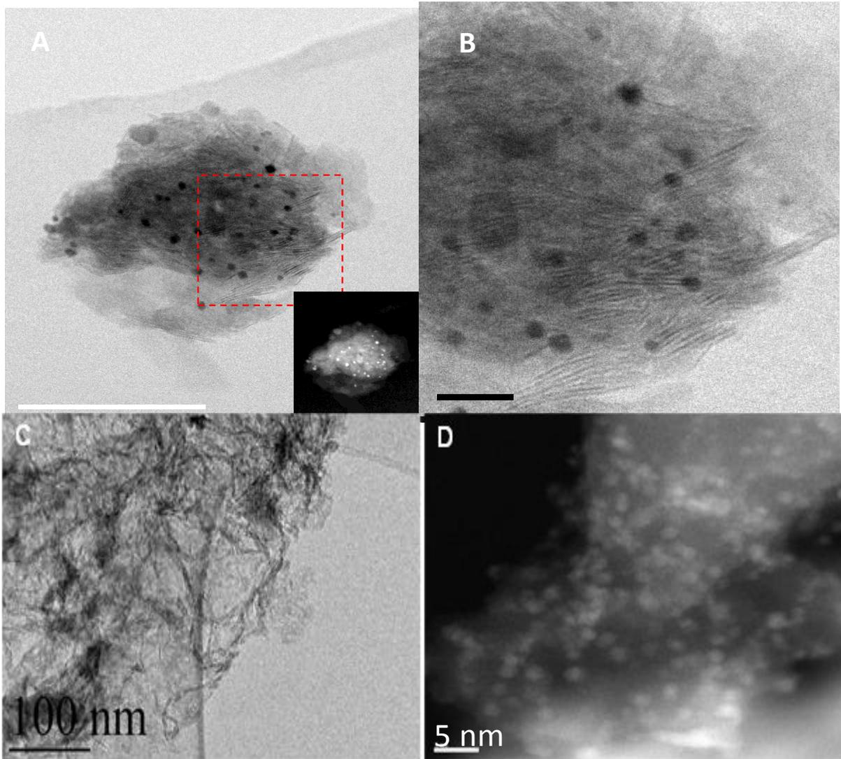
**Figure 2.** TEM images of CoCNT<sub>(10-20)</sub>/ZSM-5 (A), CoCNT<sub>(20-40)</sub>/ZSM-5 high magnification (B), MgCNT<sub>(10-20)</sub>/ZSM-5 (C) and NiCNT<sub>(20-40)</sub>/ZSM-5 (D).
