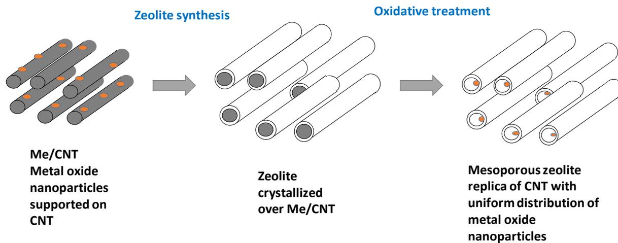
**Figure 4.** Synthesis of metal-zeolite nanocomposites using Metal/ CNT as secondary hard templates: simultaneous single-pot creating fibrous nanotube morphology, enhancement of mesoporosity and uniform introduction of active species
