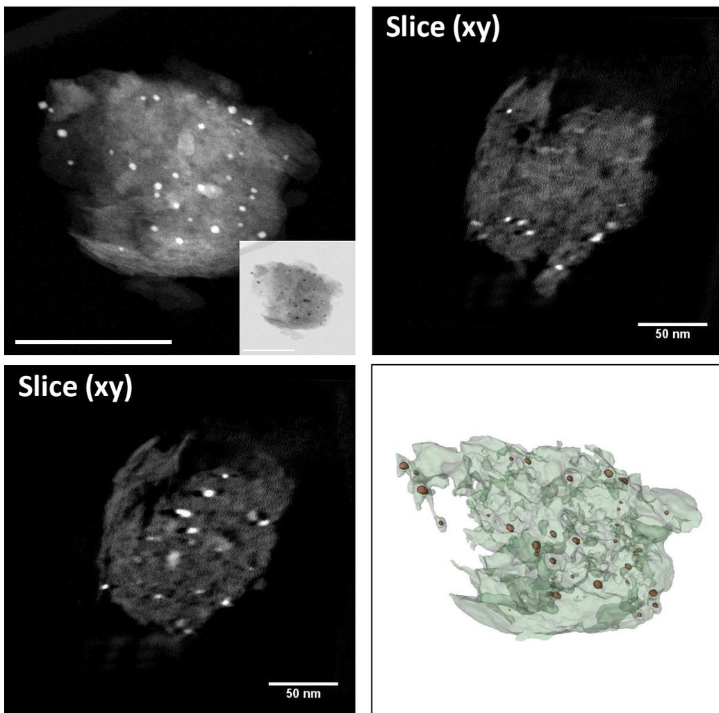
**Figure 3.** STEM-HAADF electron tomography analysis of CoCNT<sub>(20-40)</sub>/ZSM-5 clearly showing the presence of cobalt nanoparticles inside the zeolite structure
