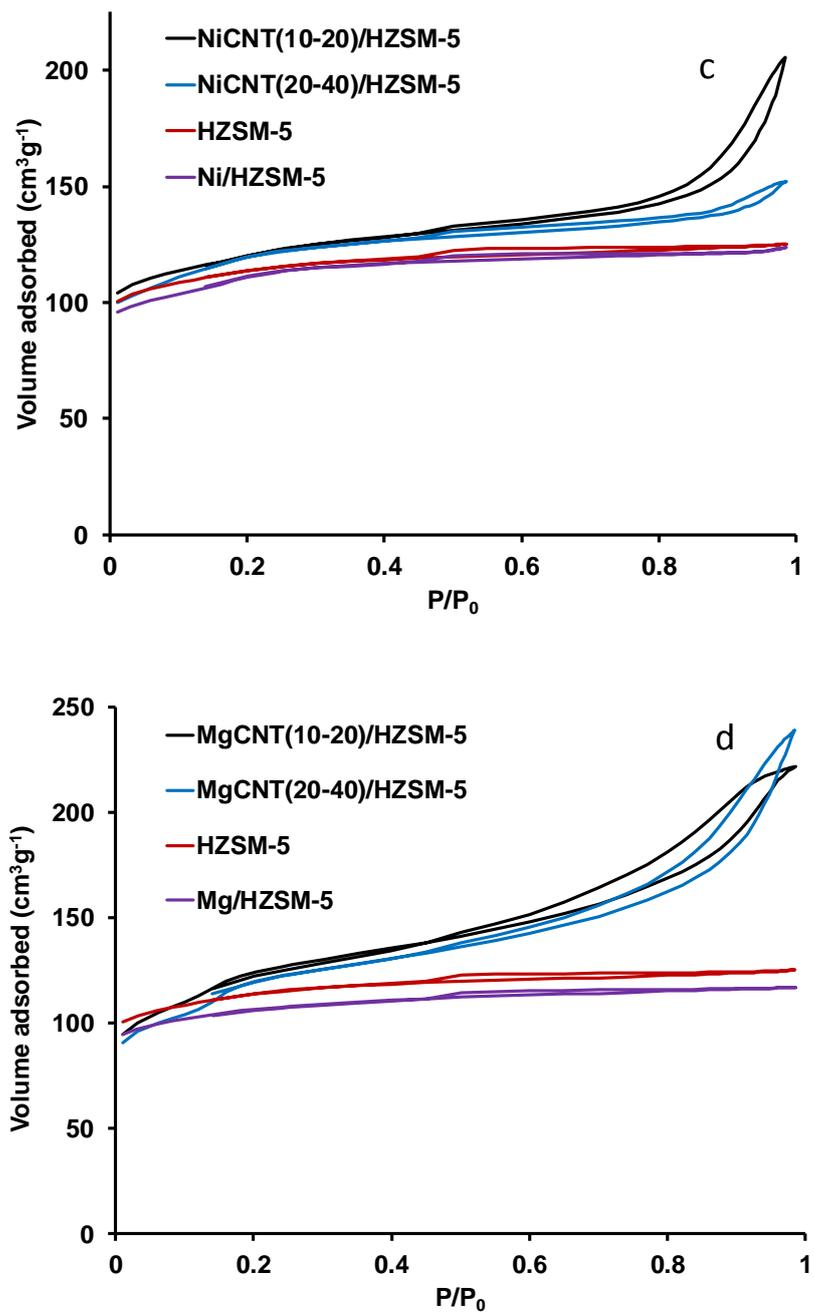
**Figure 1.** Low temperature nitrogen adsorption- desorption isotherms on the HZSM-5 zeolite synthesized with and without addition of CNT (a) cobalt (b), nickel (c) and magnesium (d) ZSM-5 catalysts. (The  $P/P_0$  region below 0.01 is not shown for clarity.)
