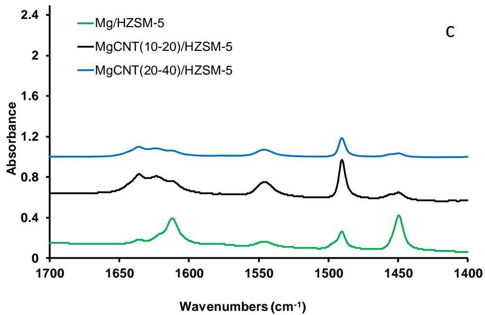
**Figure 5.** FTIR spectra observed after adsorption of Py on cobalt (a), nickel (b) and magnesium (c) zeolite nanocomposites
