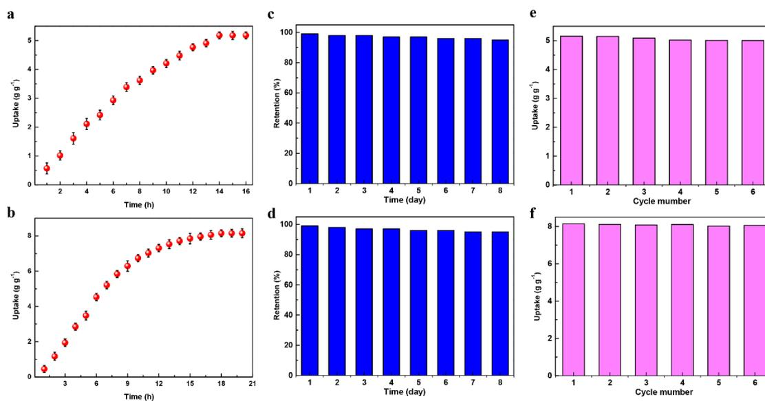
**Fig. 3 Study of iodine capture.** (a and b) Uptake of iodine of JUC-560 (a) and JUC-561 (b) as a function of exposure time at 338 K and ambient pressure. (c and d) Iodine retention of the iodine-captured JUC-560 (c) and JUC-561 (d) upon exposure to air at 298 K and ambient pressure. (e and f) Recyclability of JUC-560 (e) and JUC-561 (f) in iodine adsorption.
