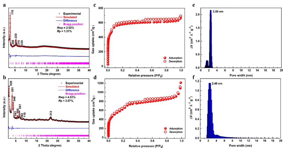
**Fig. 2** PXRD profiles and porosity. (a and b) PXRD patterns of JUC-560 (a) and JUC-561 (b). (c and d) N<sub>2</sub> adsorption–desorption isotherms for JUC-560 (c) and JUC-561 (d) at 77 K. (e and f) Pore-size distribution of JUC-560 (e) and JUC-561 (f) calculated by fitting on the NLDFT model to the adsorption data.
