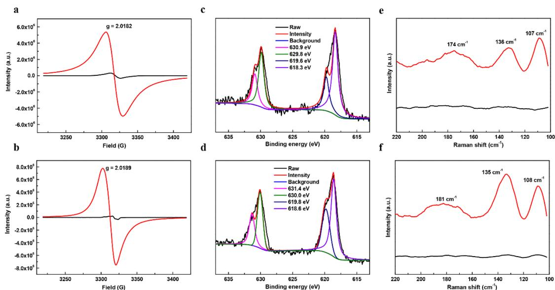
**Fig. 5 Spectroscopy study.** (a and b) EPR spectroscopy of JUC-560 (a) and JUC-561 (b) before (black curve) and after (red curve) iodine uptake. (c and d) XPS of iodine for JUC-560 (c) and JUC-561 (d) after iodine uptake. (e and f) Raman spectroscopy of JUC-560 (e) and JUC-561 (f) before (black curve) and after (red curve) iodine uptake.
