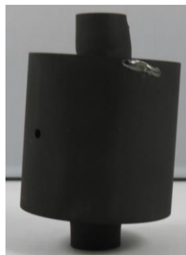
Figure 2 Photograph of the deformed punches after the flash spark plasma sintering tests.
