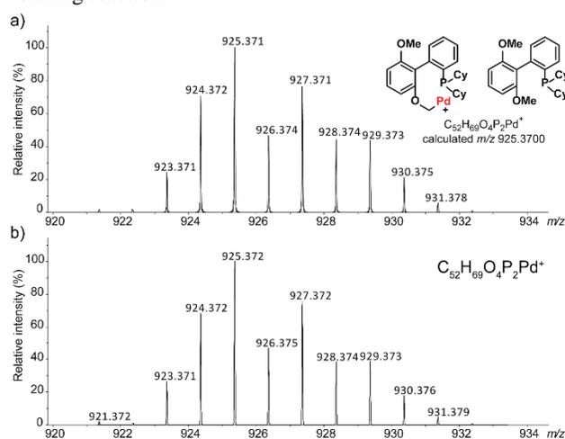
**FIGURES 1.** (a) Enlargement of the ESI(+)-FTICR mass spectrum of the crude reaction mixture showing the *m/z* 925.370 cationic palladium complex. (b) Theoretical isotopic pattern of the C<sub>22</sub>H<sub>69</sub>O<sub>4</sub>P<sub>2</sub>Pd<sup>+</sup> ion with a resolution of 60,000.
