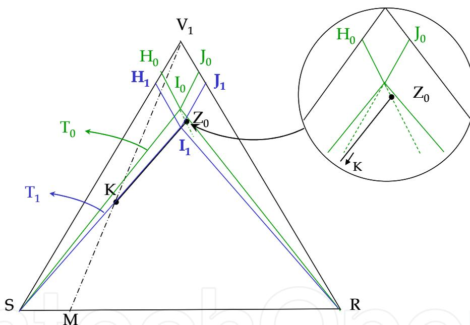
Fig. 6. Principle of crystallization by entrainment
