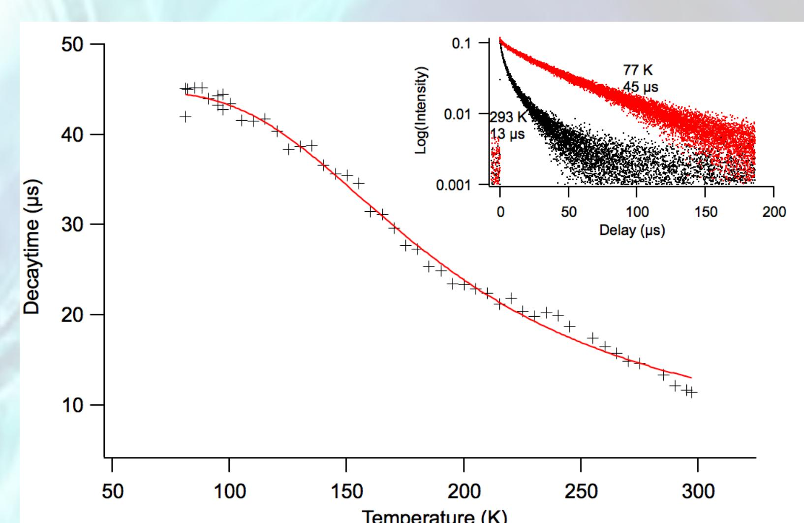
Temperature dependence of  $\lambda$  and  $\tau$  proves that the copper complexes exhibit a mixed luminescence : phosphorescence and TADF!
