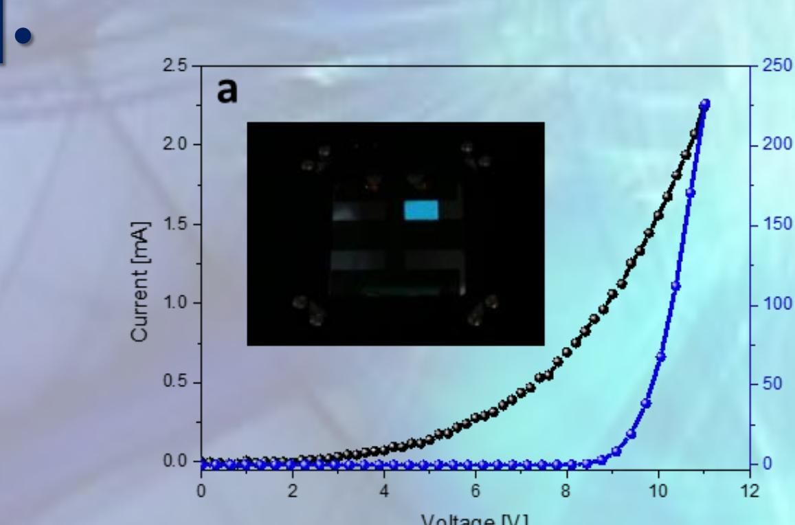
LIV-scans of devices at a scan rate of  $dV/dt = 0.2\text{V/s}$  in a voltage range of 0-11V. Inset picture shows the blue LEC during the first LIV cycle.
