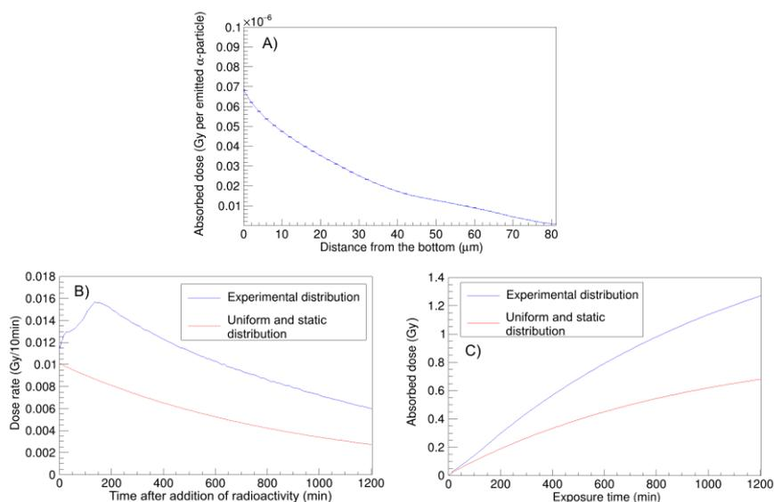
Figure 7. Dose deposited by alpha particles in a 20 μm thick cylindrical volume of water representing cell culture. A) Dose deposited per emitted α-particle according to the emission position. B) Dose deposited in 10 minutes by the experimental spatial distribution and a uniform and static distribution as a function of time. C) Absorbed dose as a function of exposure time for the experimental and a uniform and static distribution.
