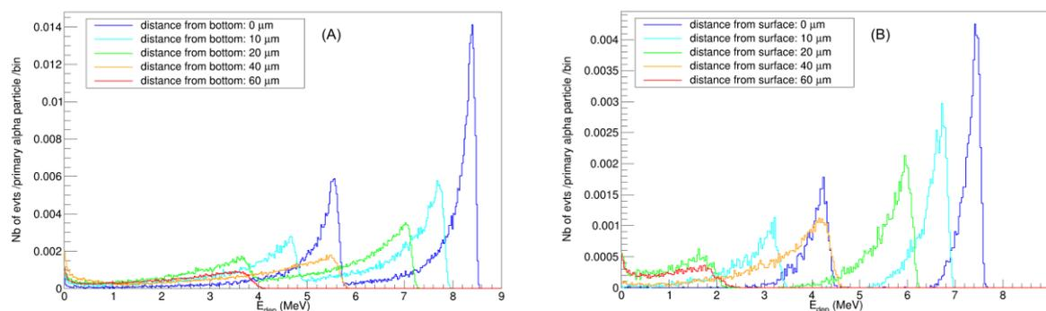
Figure 3. Energy spectra simulated in both configurations (CH1 and CH2) for alpha particles emitted from different depths.
