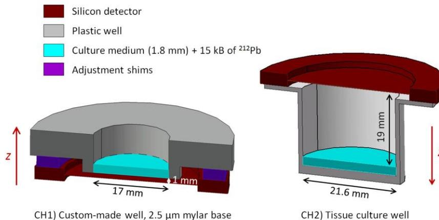
Figure 1. Cross section of the experimental setups. In the first configuration (CH1), a custom made well with a mylar base of 2.5  $\mu\text{m}$  thickness, was placed 1 mm above a silicon detector. In the second configuration (CH2), the detector was placed above a standard culture well (from 6-well plate) of 21.6 mm diameter and 20 mm height. The distance between the culture medium surface and the active area of the silicon detector was 19 mm.
