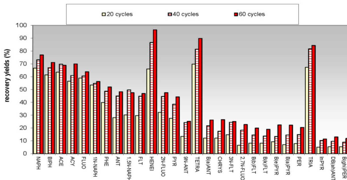
**Figure 1.** Soxhlet extraction of a mixture of spiked PAHs, nitro-PAHs and n-alkanes from 100 mg of diesel particulate matter, blown-off from a diesel particulate filter after an European NEDC driving cycle test. Extraction conditions: reflux of 120 mL methylene chloride, each cycle representing approximately 8 minutes.
