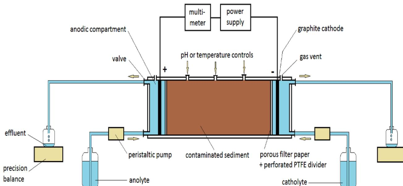
Fig. 1. Drawing schema of electrokinetic experimental set up
