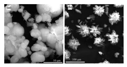
**Figure 2** SEM images of the as-synthesized samples DFZ-64C (a) and DFZ-64D (b). **Structure analysis**
