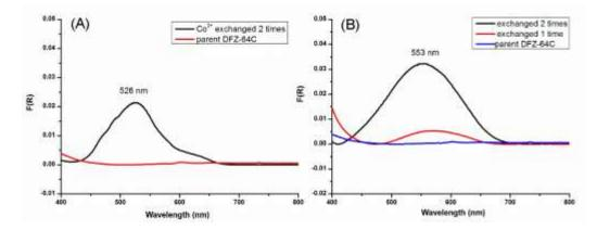
**Figure 11** The UV-VIS spectra of sample DFZ-64C after Co<sup>2+</sup> exchange in 0.05 M Co(Ac)<sub>2</sub> solution (A, 50 °C, 4h) and Cu<sup>2+</sup> exchange in 0.05 M Cu(Ac)<sub>2</sub> solution (B, 50 °C, 4h).
