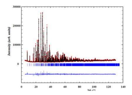
**Figure 3** PXRD diagram of DFZ-64C-LT at 20°C (Cu–Kα1 radiation; 1.5406Å) with observed (dots), calculated (solid line), Bragg reflections (ticks), and difference profiles (bottom line) obtained after Rietveld refinements.
