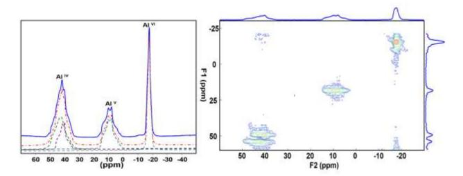
**Figure 5** 1d <sup>27</sup>Al MAS NMR spectra (left) and 2d <sup>27</sup>Al MQ MAS NMR spectra (right) of sample DFZ-64C
