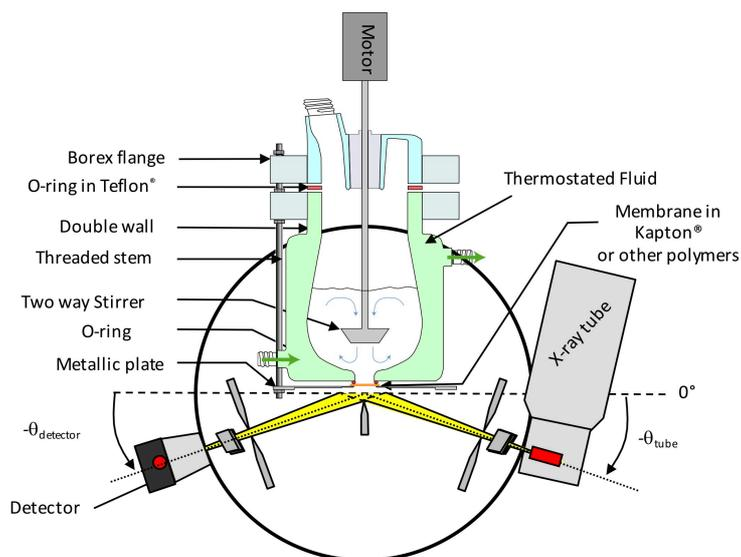
Figure 1: Schematic view of the reactor and the goniometer geometry in the In-situX<sup>®</sup> technology
