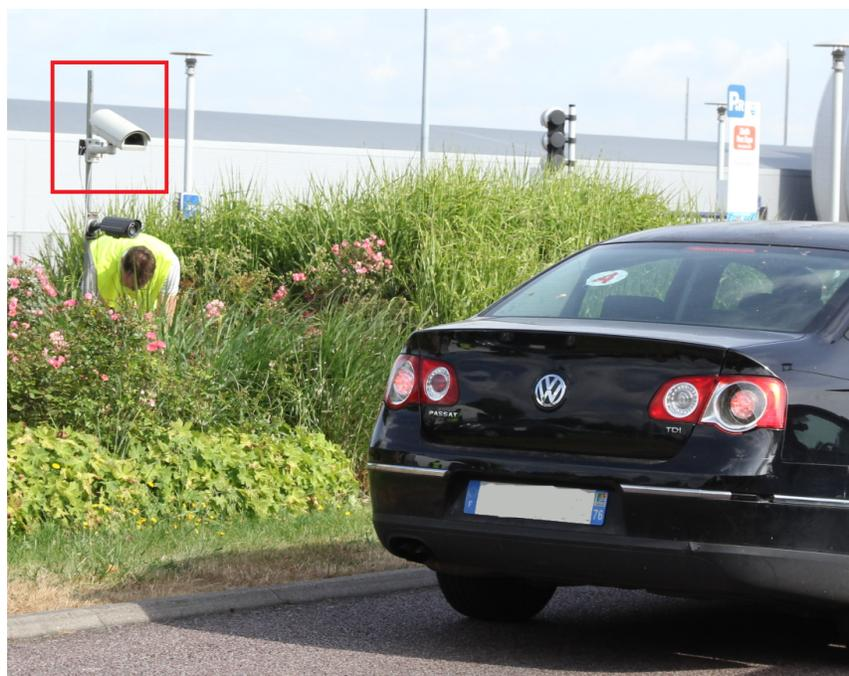
(b) Camera setup. The top camera is used for the height measurements.
