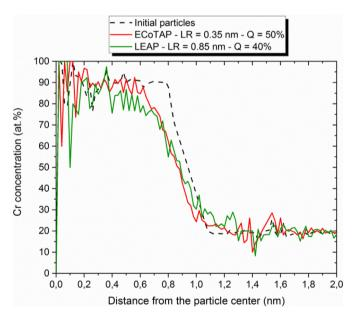
**Fig. 3.** Erosion profiles in Cr (at.%) starting from the particles centers before and after degradation of the data set. Initial Cr content of the particles is 90 at.% Cr.
