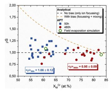
**Figure 8.** ρS as function of the Cr content (at.%) in particles 1 nm in radius measured by APT ( $X_{ij}^{CM}$ ) together with the evolution of ρS as given by equations (3) and (4).
