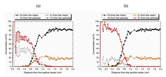
Fig. 9. Erosion profiles starting from the particle center for (a) particles having an initial Cr content of 61 at.% and (b) an initial Cr content of 84 at.%. In both case, the erosion profile was constructed on field evaporated particles after application of a LR = 0.35 nm, DR = 0.05 nm and Q = 50% (ECoTAP conditions).
