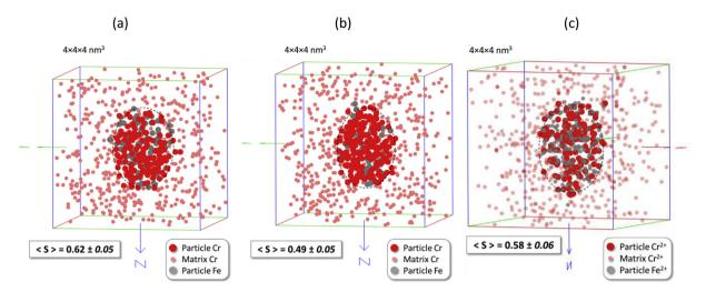
**Fig. 4.** Particle morphology after field evaporation simulation for a (a) 60 at.%Cr particle, (b) 84 at.% and (c) experimentally observed at 50 h. The average shape factor (<S>, section 3.2) is also reported. Are shown the Cr atoms from particles (big red dots), Cr atoms from the matrix (small light red dots) and Fe from particles (grey dots). (For interpretation of the references to colour in this figure legend, the reader is referred to the Web version of this article.)
