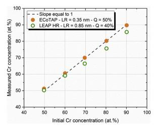
**Fig. 2.** Measured Cr concentration in  $\alpha'$  after blurring of the lattice by lateral resolution and applying detection efficiency versus the initial Cr concentration for both ECoTAP and LEAP HR. On the dashed line, the measured concentrations are equal to the initial concentrations. Uncertainties are smaller than the size of the symbols (between 0.4 at.% and 0.8 at.%). Uncertainties are smaller than the size of the symbols (-0.6-0.9 at.%).
