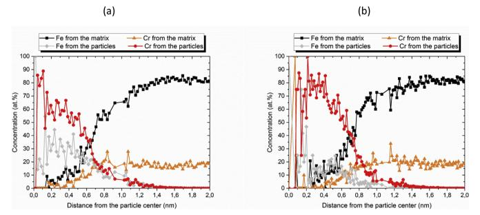
Fig. 11. Erosion profiles starting from the particle center for (a) particles having an initial Cr content of 61 at.% and (b) an initial Cr content of 84 at%. In both case, the erosion profile was constructed on field evaporated particles after application of a LR = 0.85 nm, DR = 0.05 nm and Q = 40% (LEAP HR conditions).
