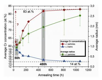
**Fig. 1.** Average Cr concentration (at.%) in the  $\alpha$  matrix and the  $\alpha'$  particles and the average radius of  $\alpha'$  particles as a function of the annealing time (h) at 500 °C. Grey rectangles highlight the conditions that will be considered in the following.
