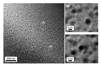
**Fig. 7.** TEM image in BF (Bright Field) conditions of Fe20Cr aged at 500 °C for 1067 h. Number density and size are identical to those measured with APT.
