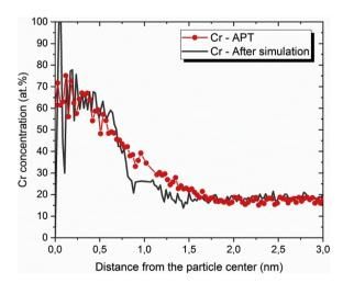
**Fig. 10.** Comparison of the Cr erosion profile for particles having a Cr content of 61 at.% as obtained after simulation of ECoTAP analysis with an experimental profile obtained in the Fe-20 at.% Cr aged 50 h at  $500\,^{\circ}$ C.
