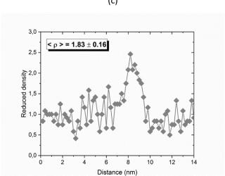
Fig. 5. Reduced atomic density profile through a particle along the evaporation direction for a simulated particle containing initially (a) 60 at% and (b) 84 at% of Cr and (c) for an experimental particle (50 h). It is also reported for each case the average reduced atomic density () [29].
