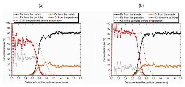
Fig. 6. Erosion profile starting from the particles center for simulated data after field evaporation simulation of particles having (a) 61 at.% and (b) 83 at.% of Cr. Atoms coming from the particles and from the matrix are distinguished. Dashed lines correspond to the Cr profiles in particles before evaporation.
