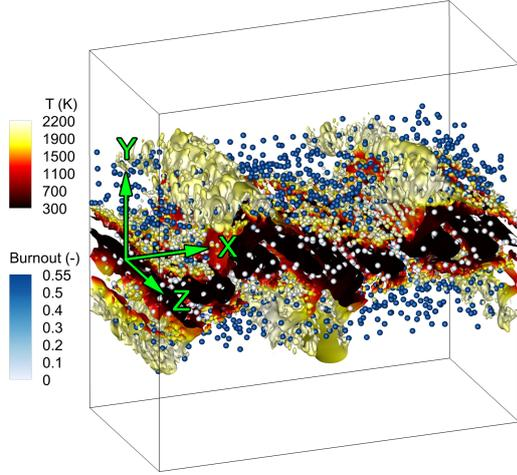
Figure 1: Instantaneous pulverized-coal particle distribution and iso- $Q$  criterion [19],  $Q = 10^5 \text{ s}^{-2}$ , colored by gas temperature. The coal particles are colored by the burnout, which denotes the ratio of the released volatile mass to the initial mass of volatile in a pulverized-coal particle.
