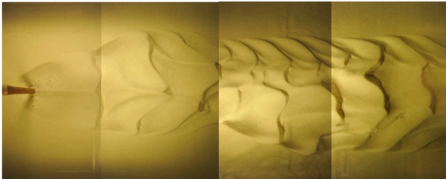
Fig. 4. Sedimentary structures downstream the cylinder; Re=42000 (Test 2)
