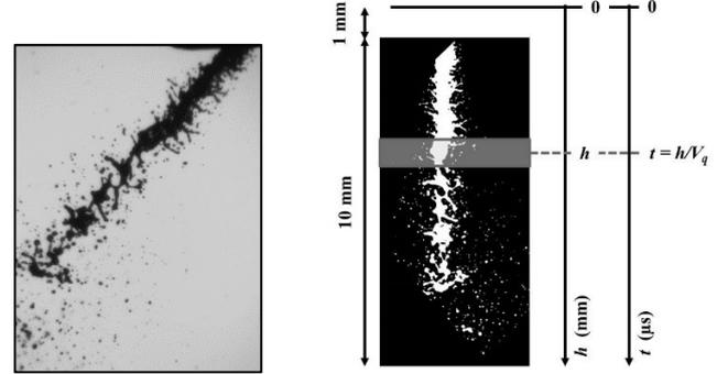
**Fig. 6:** Left – Image of the turbulent jet at 0.5 MPa (6x8 mm); Right – Local measurement of the scale distribution; The rectangle represents the analyzing window.  $h$ : position of the analyzing window, Equivalent time  $t = h/V_q$  where  $V_q$  is the jet mean velocity
