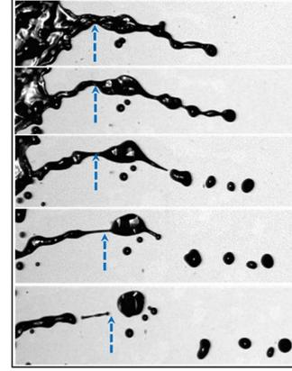
**Fig. 3:** Temporal evolution of an atomizing water ligament into air. Time gap between two consecutive images 80  $\mu\text{s}$ . Spatial resolution 10.36  $\mu\text{m}/\text{pixel}$ . The arrow indicates the point of separation used to isolate the ligament [10]
