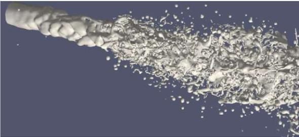
Fig. 15: Simulated atomization process of a turbulent jet. Code ARCHER
